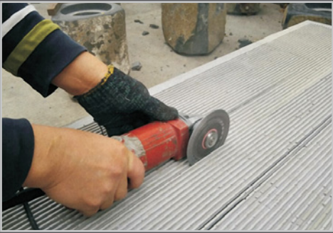
Simple cutting with angle grinder or hand saw
